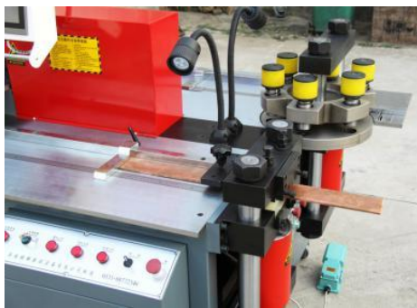
Shearing/cutting work station
